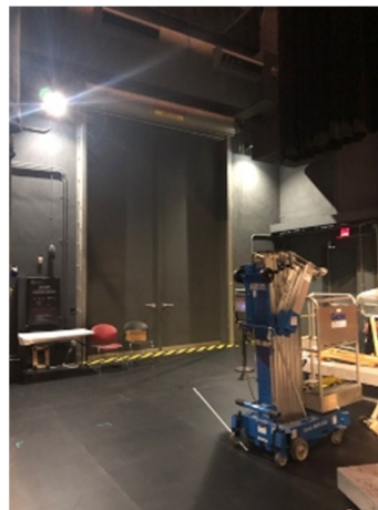
Stage Right "King Kong" Double Doors Opening measures 11'-6 3/4" wide x 17'-3 1/2" tall
